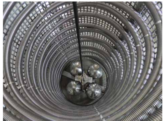
view from above of the self-limiting heating cable routed in a corrugated stainless steel tube and the Ex floating electrode
