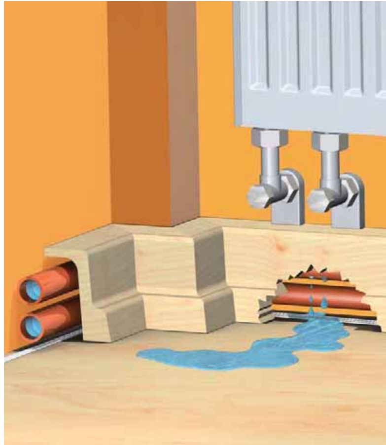
Use of a twin electrode for leakage detection of electrically conductive heating water under a skirting board behind which pipes are routed
